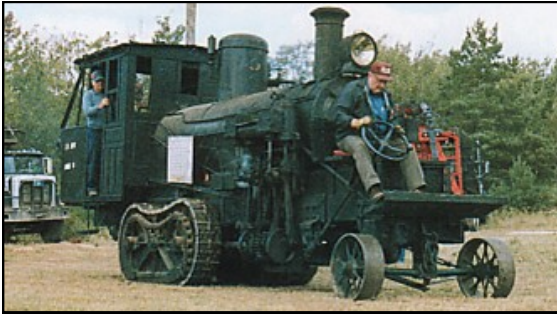
Steam log hauler made by Phoenix Manufacturing Company of Eau Claire, last known operational Phoenix in the state..
