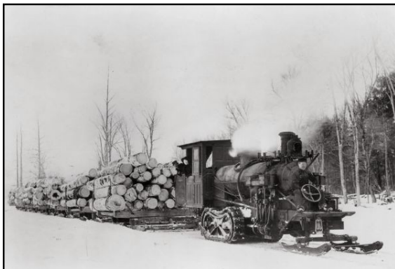
Steam log hauler made by Phoenix Manufacturing Company of Eau Claire, pulling loaded skids through snow. Rice Lake lumber camp, overland spur, ca. 1914. Wisconsin Historical Society.
